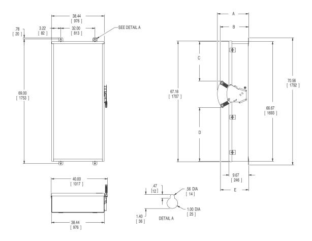
No knockouts in enclosure. Dimensions shown in inches and millimeters ( ). Dimension shown accurate to  $\pm\,1\!\!/\!_{2}$  inch.
