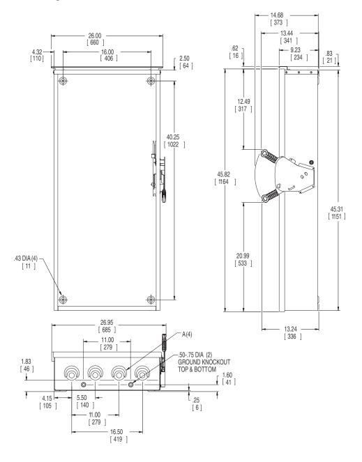
Dimensions shown in inches and millimeters ( ). Dimension shown accurate to  $\pm$  ½ inch.
