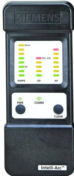
5. The communication LED will start blinking after the handheld establishes communication with the base unit. The LED will continue blinking as long as the handheld maintains communication.
