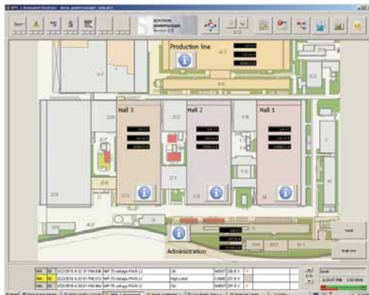
Plan overview provides energy usage per building
