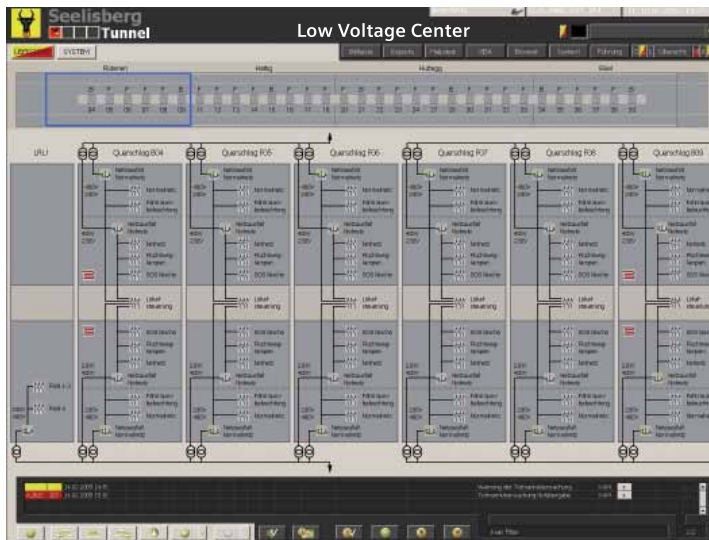
Simple one line diagram displaying low voltage system information
