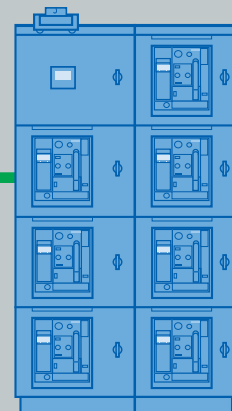
Low Voltage Switchgear
