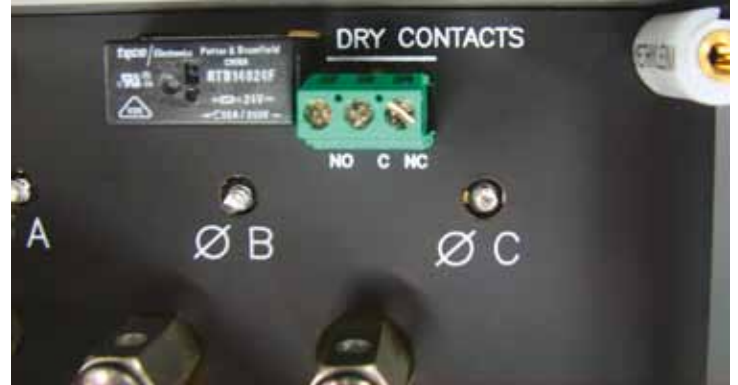
Figure 8: Dry Contact Pin Configuration
