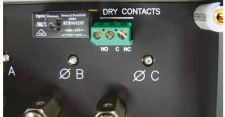
A typical application using a Normally Closed configuration would connect to one set of the N.C. and Common terminals. During an inoperative condition, the SPDs dry contact would change state from normally closed to open. We generally suggest the Normally Closed configuration because it will detect a wiring defect, such as cut wire(s), where N.O. will not.
