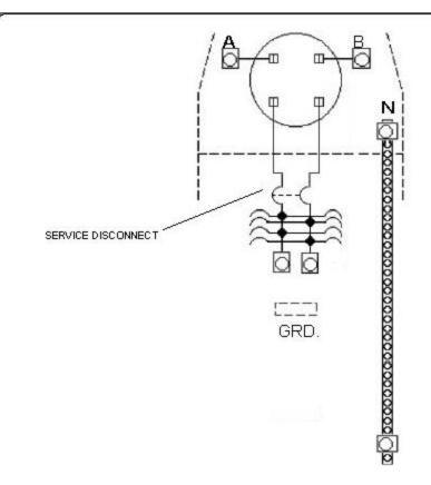
Short Circuit Current Rating (Watthour Meter not included in short circuit current rating) This panelboard has a maximum short circuit rating of 10,000 RMS symmetrical amperes, 240 volts maximum with breakers listed below installed.
