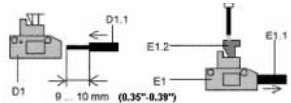
Connecting and disconnecting wire
