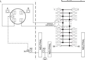
SHORT CIRCUIT CURRENT RATING (WATTHOUR METER NOT INCLUDED IN SHORT CIRCUIT RATING) THIS PANELBOARD HAS A SHORT CIRCUIT CURRENT RATING OF 22,000 AMPS RMS SYMMETRICAL, 120/240 VAC.
