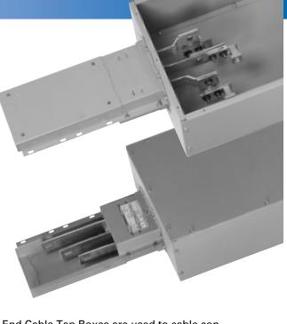
End Cable Tap Boxes are used to cable connect incoming service to BD Busway. When mounting busway sections flush against a wall or a flat surface, the busway must be mounted with the offset to the right of the installer. This will permit the end cable tap box to mount flush against the wall. BD Busway end cable tap boxes are provided with robust wire bending space to make pulling cables less labor intensive.
