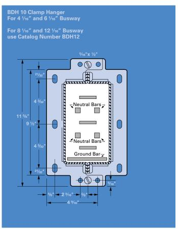
Three bolt holes in both ends of Hanger allow half the hanger to be adjusted to fit two BD Busway casing sizes (4  $\frac{1}{16}$ " and 6  $\frac{1}{16}$ "). Hanger rods and brackets are supplied by installer.
