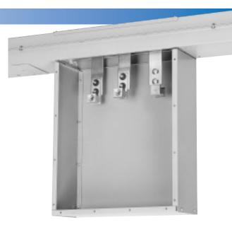
Center Cable Tap Boxes are used to cable connect incoming service to BD Busway. Center cable tap boxes are a convenient way to feed power at an intermittent point along the busway system to distribute power in two separate directions. BD Busway center cable tap boxes are provided with robust wire bending space to make pulling cable less labor intensive and are built to easily interchange with a standard 10'-0" plug-in straight length.
