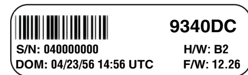
Figure 1: ACCESS 9340/9360 Meter Label Example
