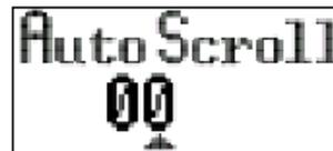
3. Enter your desired time lapse by pressing the Up Arrow button to increment and the Down Arrow button to decrement the time lapse between each screen display. Press the Select button to accept the change. Enter your password at the prompt if required and press the Select button.
