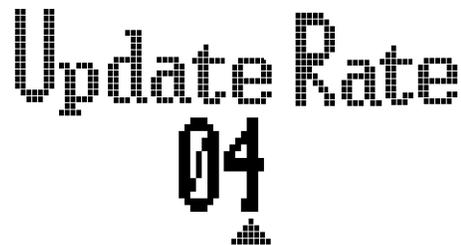
3. Enter your rate by pressing the Up Arrow button to increment and the Down Arrow button to decrement the time lapse. Press the Select button to accept the change. Enter your password at the prompt if required and press the Select button.
