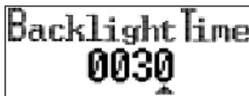
3. Enter your desired time delay by pressing the Up Arrow button to increment and the Down Arrow button to decrement the time lapse. Press the Select button to accept the change. Enter your password at the prompt if required and press the Select button.
