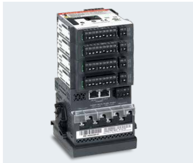
Bottom view of 9410 meter unit, showing dual Ethernet port and RS-485 communication port connectors, configuration switches and 4x expansion I/O modules.
