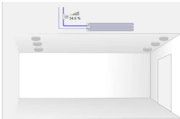
Sample presentation of a chilled/heated ceiling application on the Desigo CC management station.
