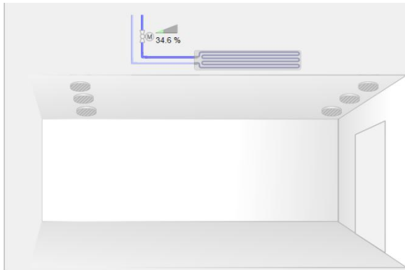
Sample presentation of a chilled ceiling application on the Desigo CC management station.
