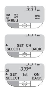
To change 1st ON time for CH press SELECT, time will flash, change times by using \( \times +l-\subset, \) when desired time is in the display press ENTER display will show \_\_\_\_\_\_
