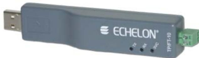
*The Echelon U10 USB Network Interface – TP FT10, needed for NK823x*
