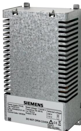
This power supply can be installed in fire control panels or in additional housing intended for this purpose. When it is used in additional housing, the power supply must be monitored by the fire control panel.
