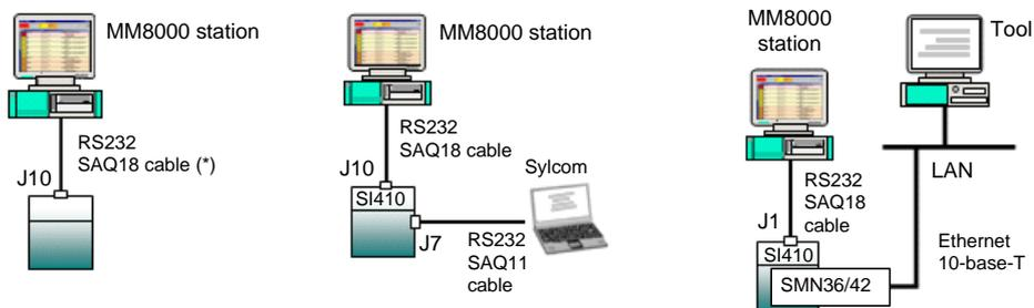
(\*) The small printer circuit on one end of the cable is labelled SMQ18.
