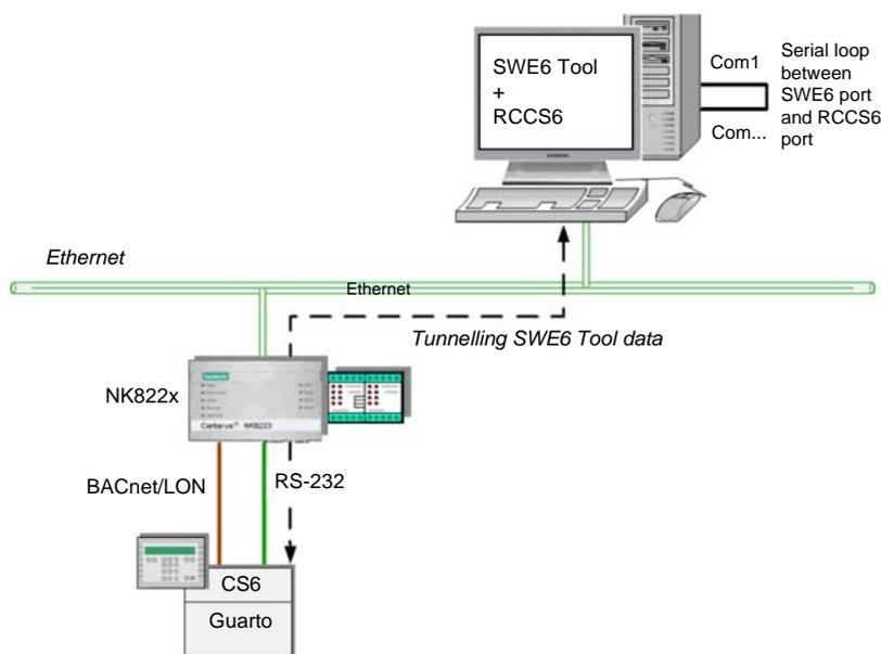
Tunnelling for remote CS6 configuration
