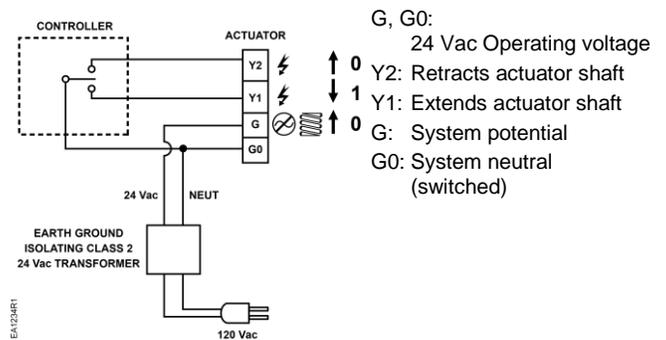
**Figure 11. SSD81.5U Floating Control SR Neutral Switching Applications.**
