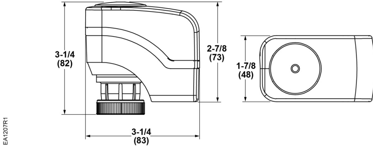
Figure 18. SSD61U/SSD81U Actuator in Inches (Millimeters).
