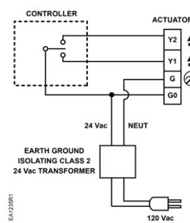
**Figure 9. For Non-Triac Driven Controllers.**
