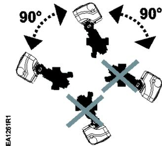
Figure 2. Acceptable Mounting Position with Valve.
