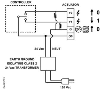
**Figure 10. For Triac Driven Controllers, (TEC, DXR, and Others).**
