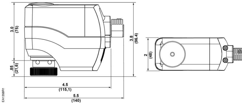
Figure 19. SSD61.5U/SSD81.5U Actuator Dimensions in Inches (Millimeters).
