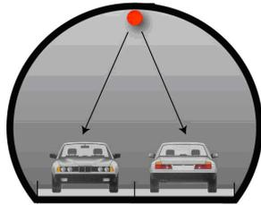
Fig. 9 Tunnel with a width < 10 m and one sensor cable
