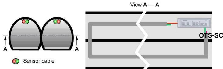
Fig. 19 Partial-redundant installation with one Switch-Controller
