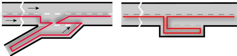
Fig. 11 Cabling in entrances and emergency bays
