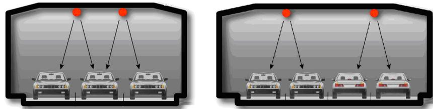
Fig. 10 Tunnel with a width > 10 m and two sensor cables
