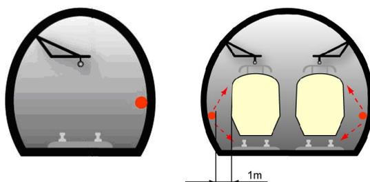
Fig. 12 Single-tracked and double-tracked tunnels
