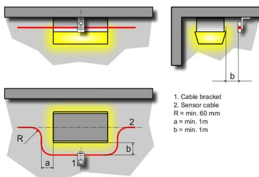
Fig. 7 Installation around lamps
