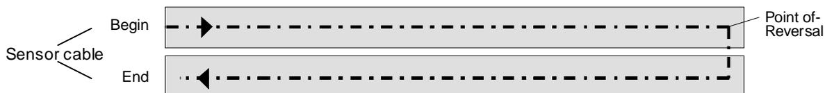
Fig. 16 Monitoring of two tunnel tubes with one sensor cable
