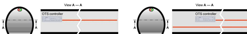
Fig. 17 Optimally vs. not optimally suited controller position
