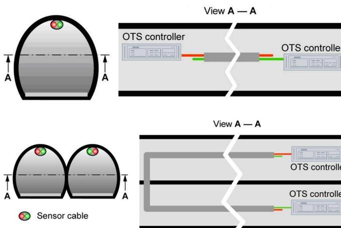
Fig. 18 Redundant system with one sensor cable
