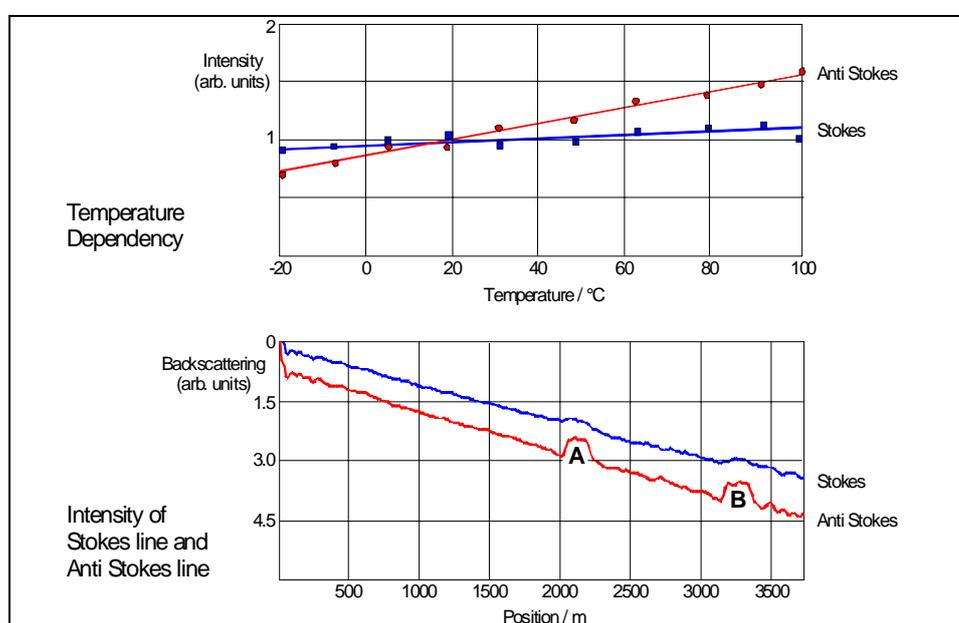
Fig. 22 Raman backscatter curves
