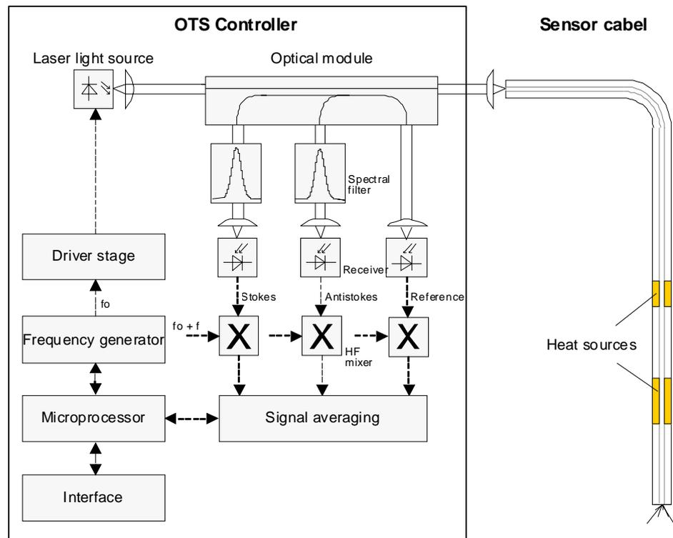
Fig. 21 OFDR- Raman temperature measurement system
