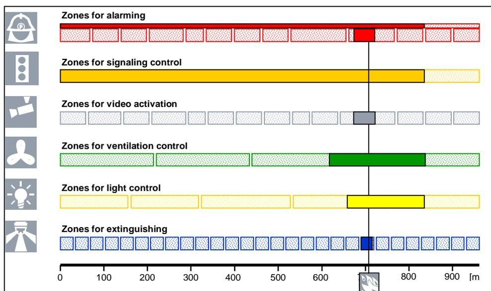
Fig. 6 Activated controls based on zones and fire location
