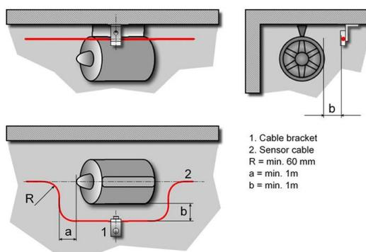
Fig. 8 Installation around fans
