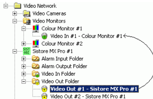
Fig 22 Connecting SISTORE to monitors
