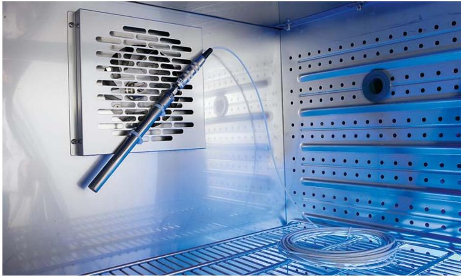
The customized sensor measures and monitors the temperature within refrigerators.
