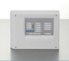
XC10 control panels combine fire detection and extinguishing – by acting as an interface between the two: After receiving a fire alarm from the connected detectors, the combined XC10 panels trigger the extinguishing system. They can be used for single- or multi-sector applications. Additional repeater terminals allow remote control of the XC10.
