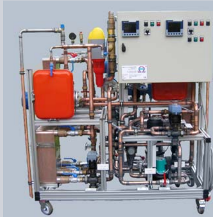
Test bench for brine-to-water heat pumps with capacities up to 32 kW
