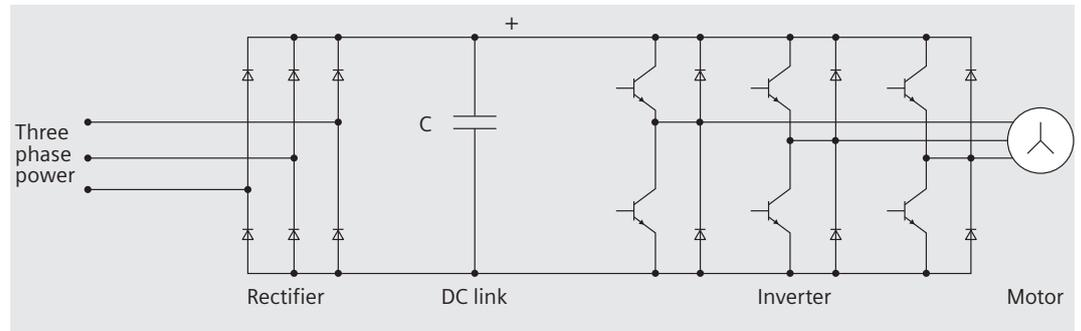
Power flow in a VSD single line diagram
