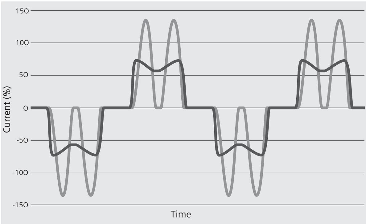
**Current waveform of a typical 6-pulse VSD vs. the SED2**
