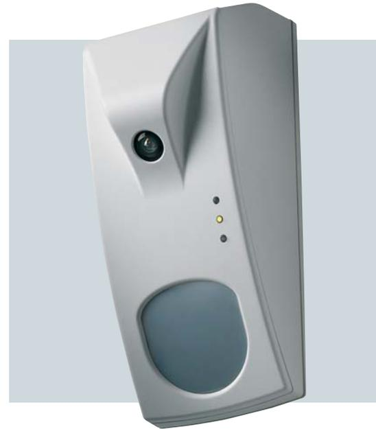
The Eyetec dual motion detector requires a minimum of 0.5 lux light conditions. Below this level, Eyetec works as a high quality 15 m PIR detector with antimask – alarm are then not restricted to a defined area or direction of movement.
