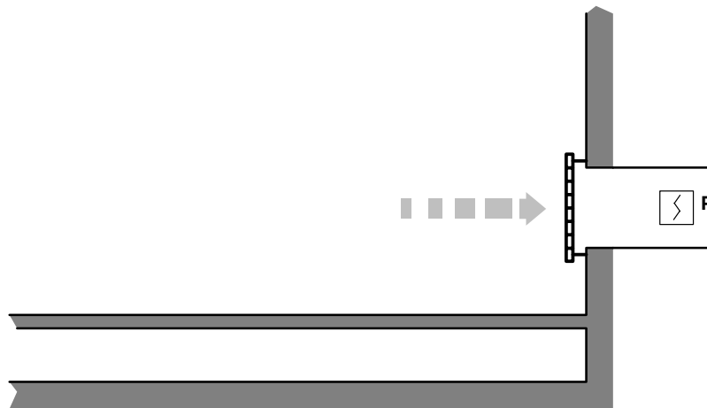
Fig. 36 Return air vents in the wall near the floor: In addition to the detectors on the ceiling, monitoring of the return air duct with the air-sampling unit ASD-duct detector unit is recommended
