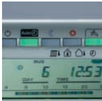
Simple operating mode selection at the push of a button
