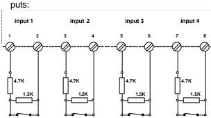
• 4-NO supervised input module (DF8046) - Provides 4 balanced, normally-open in-
