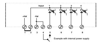
4-NC supervised input module (DF8045) - Provides 4 balanced, normally-closed inpute:
