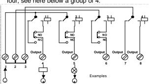
• 8-input module (DF8040) - Provides 8 digital inputs with galvanic isolation, see below a group of 4 inputs
