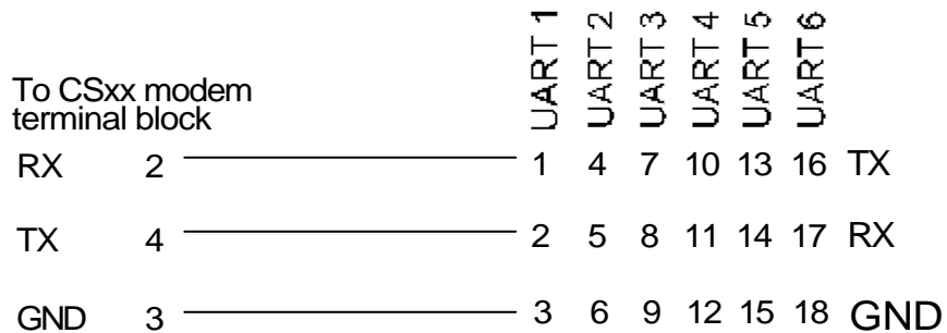
Fig. 13 GW-21 to CSxx subsystem (screw terminal block)
