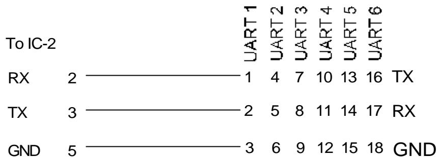
Fig. 14 GW-21 to CMX link (screw terminal block)
