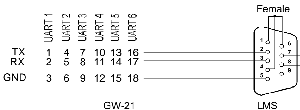
Fig. 10 Connection to 9 pin D connector (screw terminal block)
