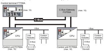
The FC700A is a modular 4 − 16 Loop fire alarm control panel for use with Synova<sup>TM</sup> analogue addressable devices. The FC700A can be self-contained or operate on a network of up to 16 panels, user terminal or BMS gateways.
