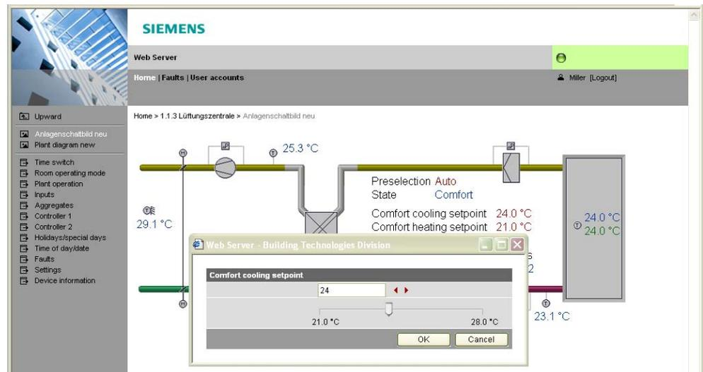
Plant diagrams also allow for integrating additional data such as links to plant, function, and maintenance descriptions or data sheets. Integrating external links allowing users to navigate to several plants is possible also. In addition, plant diagrams even allow users to integrate current webcam pictures.
