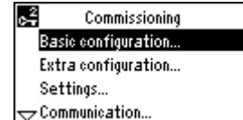
4. Select submenu "Basic configuration". Select the plant type / basic type and the position of the option modules.
