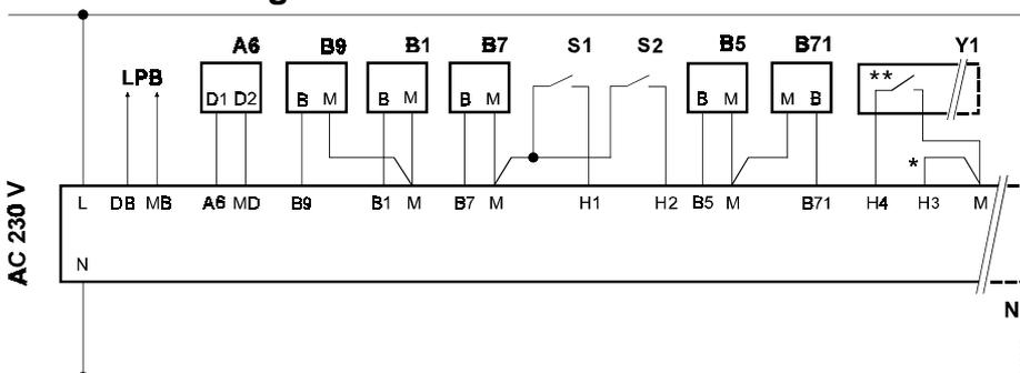
Basic connections on the low voltage side
