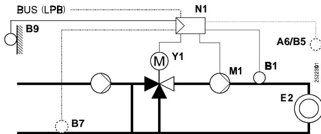
**Plant type 2:** space heating with own boiler (on/off control, acting on burner)
