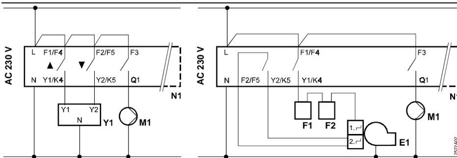
Basic connections on the mains voltage side
