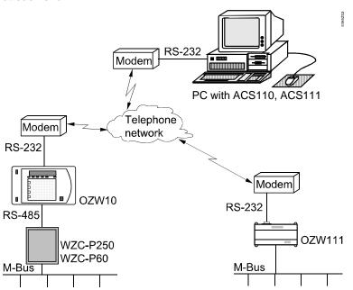
For detailed information about the RS-232 cables, the null modem, modems, M-bus and RS-485, refer to the Basic documentation CE1P5361en.
