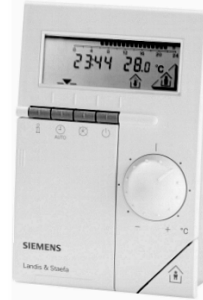
QAW70 room unit, with room temperature sensor, time switch, setpoint adjustment and readjustment of the room temperature setpoint (setting knob)
