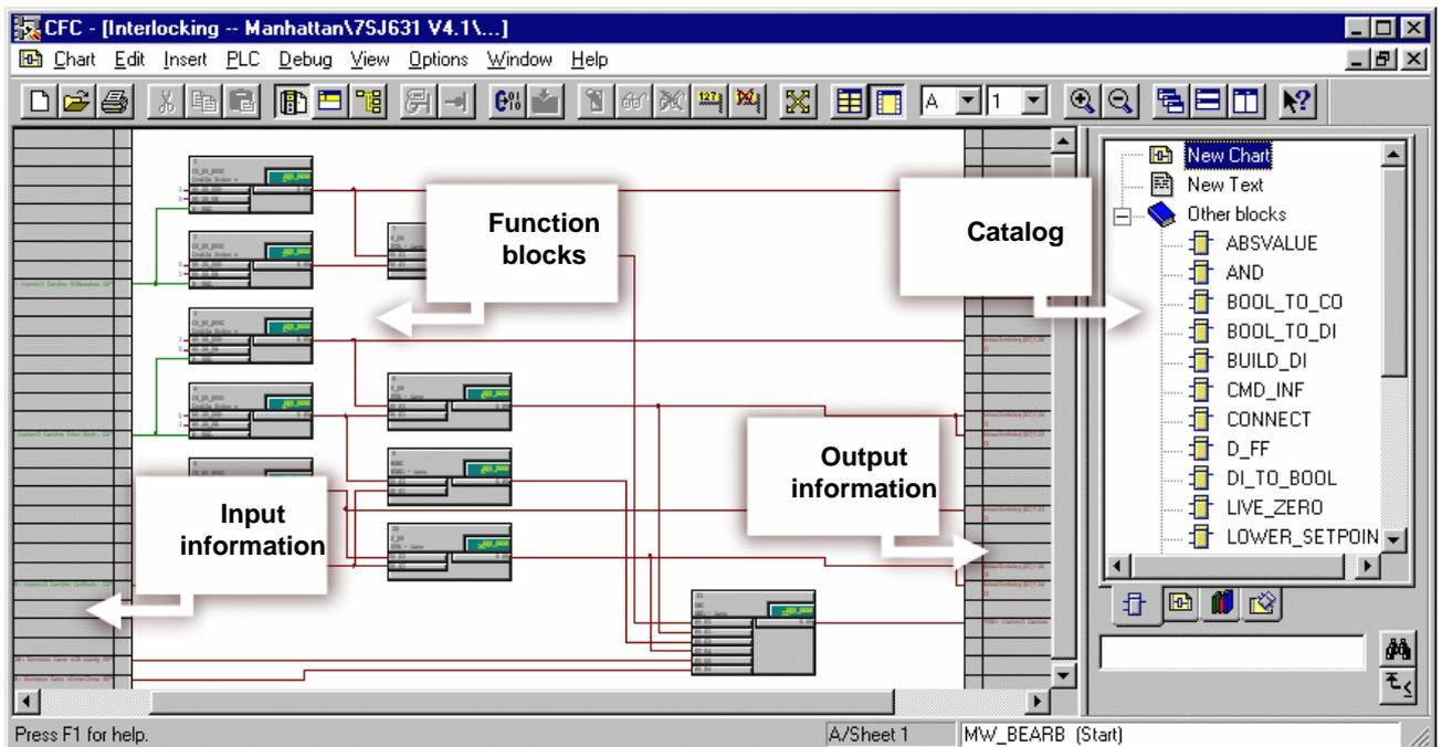
With **DIGSI 4 CFC** you can create logic functions without programming.
