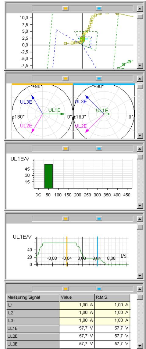
The five views in **SIGRA 4** starting from the top: locus diagrams, vector diagrams, bar diagram, curve and tabular display of values.
