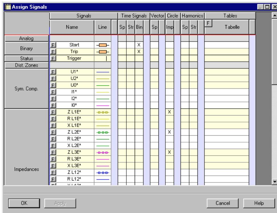
You use the signal matrix to assign signals to individual diagrams.
